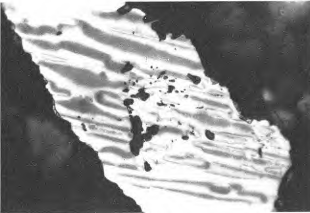
Fig. 8. Large multidomain grain with lamellae-shaped domains. The cluster of nonmagnetic inclusions within the ore grain produces extremely small domains with presumably pseudo-single-domain behaviour. The diameter of the figure is 120 \mu\text{m}
